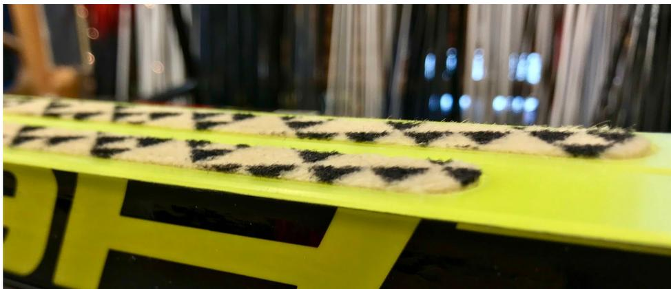
*A close inspection of Fischer's Skin patterns shows variable depth from front to back and offset placement.*
